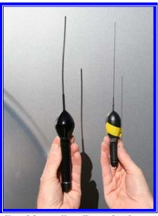
The new X model pop-off satellite archival tag (right) that will be used in 2008 is roughly half the size of its predecessor and will allow smaller fish to be tagged.
